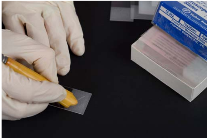
A sample is collected by gently rubbing the surface of the object over the frosted end of a microscope slide.
