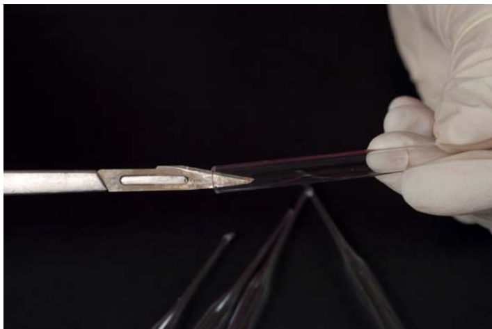
The tubular end of the pipette makes a useful funnel to collect the sample and push towards the capillary end.
