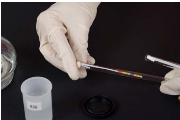
Once the sample and indicators have been placed in the pipette, the tubular end is sealed with modeling dough such as Plasticine . Then the sample in the capillary end of the pipette is heated using the alcohol burner, to free the combustion vapours.
