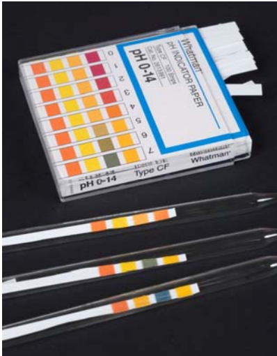
The color of the strip in the pipette is then compared to the pH reference scale provided with the strips. Here, front top to bottom : pH 4.0, pH 6.0 and pH 9.0 (reading on the back of the box).
