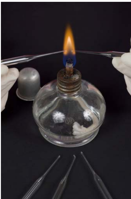
The capillary end of Pasteur pipettes can be rapidly flame-sealed.
